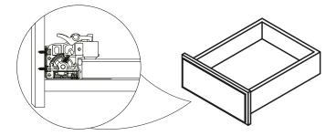
3) Please put the drawer flat on the slide and close the drawer completly. When the slide be connected with the connecting link, then the installation to be finished.
