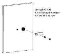
4.Install L-type strike plate using supplied
